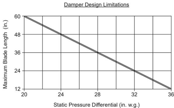
This damper's design at a blade length of 60" has a maximum allowable blade deflection of  $L / 360$  for the static pressure indicated on the chart. At reduced blade lengths, higher static pressure limits can be attained without sacrificing damper operating performance characteristics.
